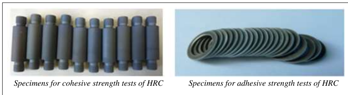
Figure 1 Specimens to determine the strength properties of HRC layers
