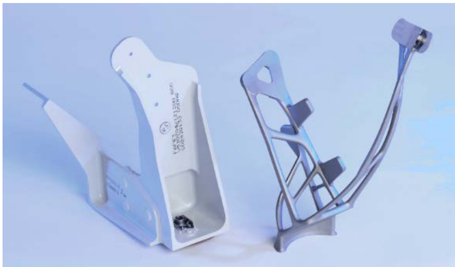
Figure 1. Secondary Structure (Bracket) developed by Premium Aerotec GmbH. Conventional design (milling plus riveting) compared with topologically optimized design developed for the Additive Manufacturing (53% weight saving, 40% cost saving).
