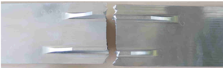
Figure 1. WEND specimen in an alloy showing a straight path after completion of the fatigue test.
