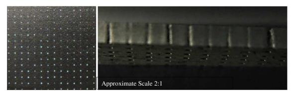
Figure 1. Top view and cross section of a laser micro drilled plate [Pictures by Airbus].
