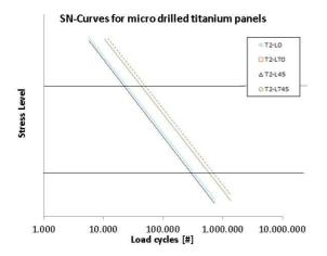
Figure 2. Initial test results from the test matrix.
