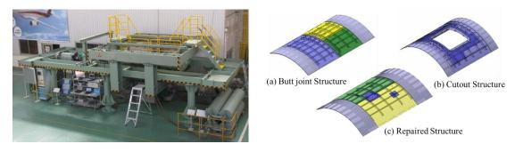
Figure 2. Fuselage curved panel test setup. Figure 3. Curved panels for damage tolerance evaluation.
