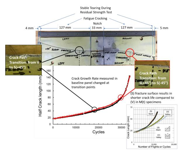
*Figure 2: Phase 1 test results of baseline panel showing crack surface morphology and effect on fatigue crack growth.*
