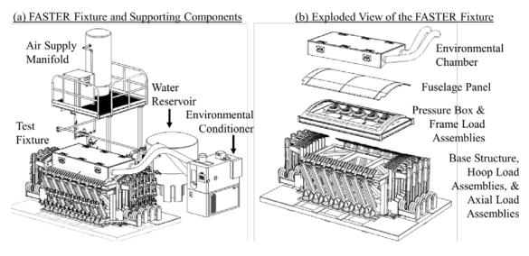
Figure 1. Full-Scale Aircraft Structural Test Evaluation & Research (FASTER) fixture
