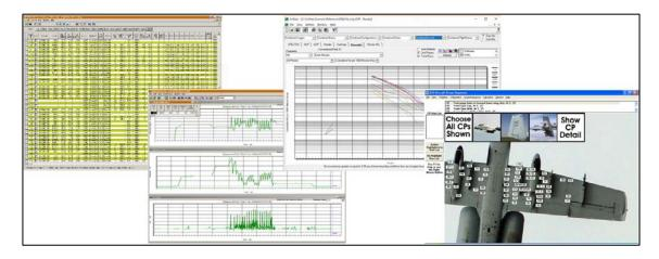
Figure 1. Software tools developed for A-10 flight data processing, maneuver spectra generation, and stress sequence development.
