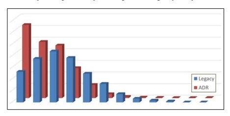
Figure 2. Histogram of landing sink rate design assumption (Legacy) and as recorded (ADR).
