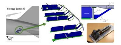
Figure 3. The certified 787 aft galley diagonal additively manufactured fitting.
