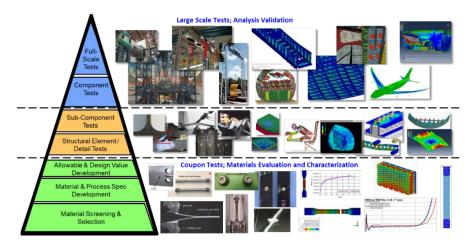
*Figure 1. The structural test pyramid, with a smarter level of certification testing.*
