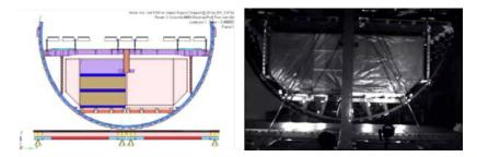
Figure 2. Fuselage drop simulation (left) and test (right) demonstrating 787 airframe crashworthiness.
