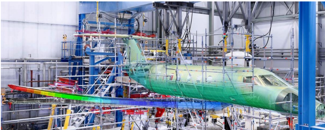
Figure 1. Full-Scale Fatigue Testing
