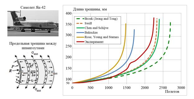
Figure 8.1.1 Comparison of computed and experimental results of longitudinal crack growth between ribs obtained using the various buckling models (Yak-40 airplane)
