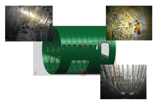
Figure 8.2.1 Fuselage full-scale section of MC-21 -300 airplane used for damage tolerance tests followed by residual strength tests
