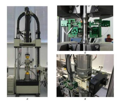
Figure 3.4.1 Servohydraulic test system Instron 8850 (a). Dual-axis strain sensors installed on the sample for testing at normal (b) and high temperatures (c)
