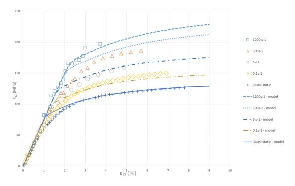
Figure 4.5.1 Experimental and predicted inplane shear loading diagrams
