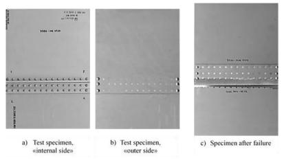
Figure 9.4 Specimen of longitudinal fuselage skin joint made of 1163RDTV alloy
