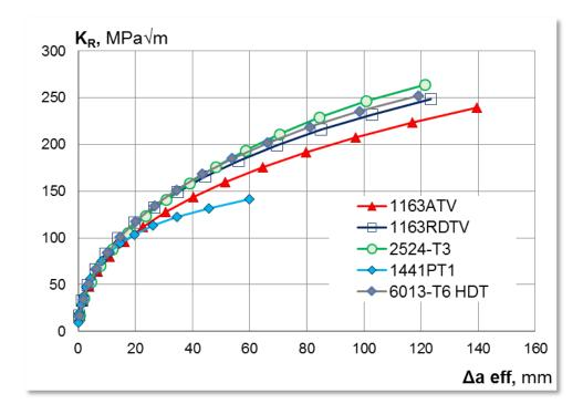
Figure 3.1.8 R-curves of the fuselage skin material
