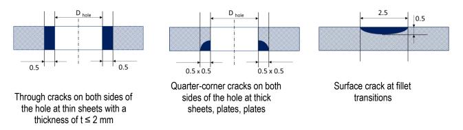
Figure 2.1 Typical damages or initial manufacturing defects recommended for considerations while analysis
