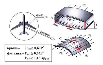
Figure 2.2 Airframe regulated damages
