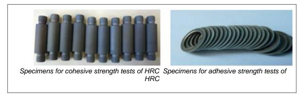
Figure 11.1.1 Specimens to determine the strength properties of HRC layers
