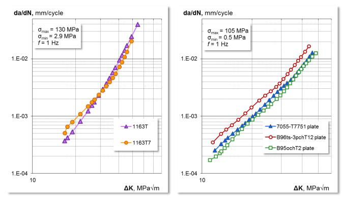
Figure 3.1.3 Crack growth curve of the wing lower surface material
