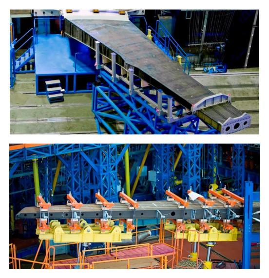
Figure 4.1 Full scale composite structures under experimental studies at TsAGI on structural integrity
