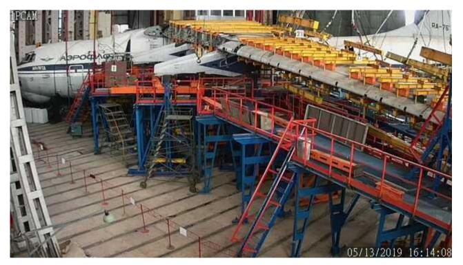
Figure 10.1.2 IL-76MD Fatigue tests of aircraft structure elements in lab
