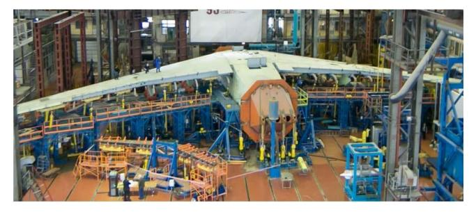
Figure 10.1.3 Static test of wing - central fuselage section with main landing gear in TsAGI lab
