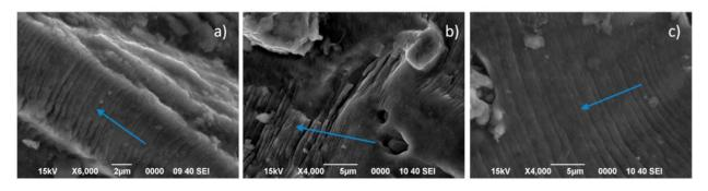
Figure 3.2.1 SEM fractographs of samples (a) S1, (b) S2 and (c) S3. The blue arrow indicates the direction of crack growth.
