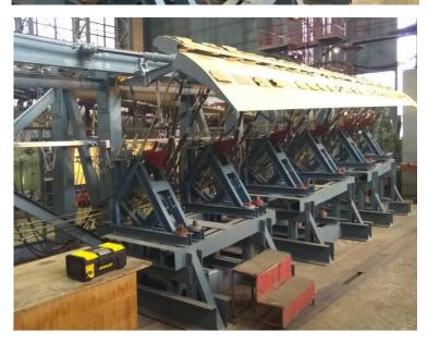
Figure 10.2.2 Test of IL-112 flap mechanisms for operation & functionality
