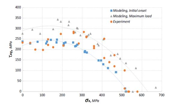
Figure 4.6.1 Biaxial failure envelope for [90/ $\pm$  30/90] E-glass/LY556 epoxy laminate under combined  $\sigma_x$  and  $\tau_{xy}$  stresses
