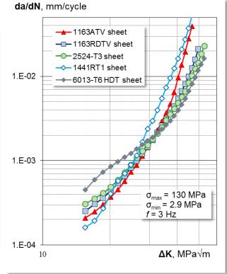
Figure 3.1.5 Fatigue curve of the <u>fuselage</u> skin material
