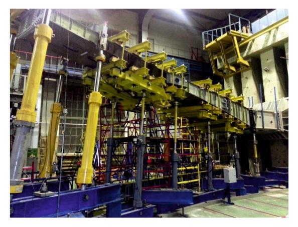
Figure 6.2 Fatigue tests and residual strength test of composite wing box structures
