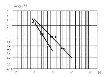
Figure 11.2.2 Influence of vibration loads on the thermal fatigue durability of ZhS6U alloy: x - 2%;  $\bullet - 1\%$ ,  $\blacktriangle - 0,5\%$ ;  $\circ$  – with imposed vibration.
