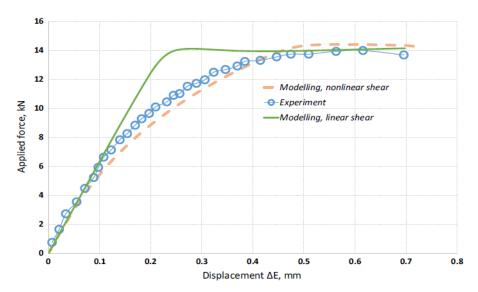
Figure 4.6.3 Experimental and predicted loading diagrams with linear and nonlinear shear stiffness
