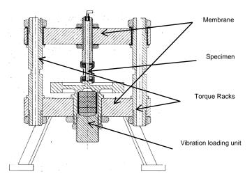
Figure 11.2.1 P926 test rig allowing independent axial cyclic loading at various levels in combination with thermal stresses
