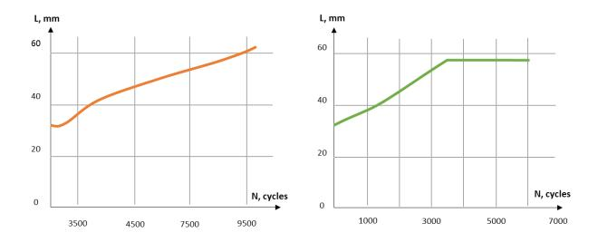
Figure 8.2.2 Crack growth in cargo door edge obtained from test
