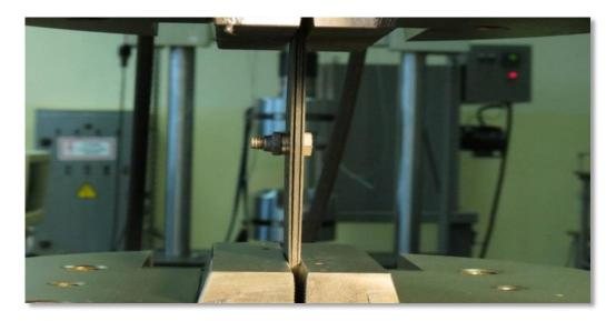
Figure 4.3 Photo of the tested strip CFRP specimen installed in the test rig
