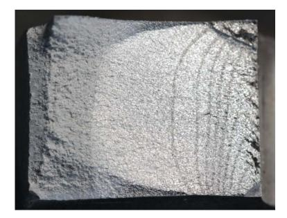
Fig. 12 - Evolution of the crack front in Cold Expanded pin loaded hole, as evidenced by marker loads.
