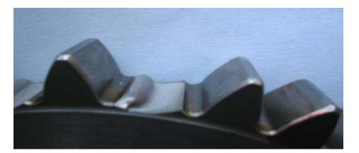
(a) Root Failure (RF)
