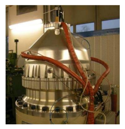
Fig. 11 – Dedicated planetary rig, for testing planet gear bearings.
